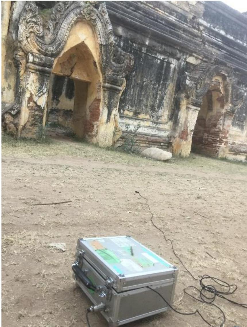
Figure 1.4 Microtremor survey at site no 7.
